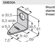
3032723 Mounting bracket, rectangular, stainless steel, for sensors with 30mm
