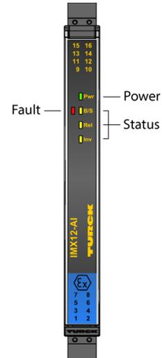
The IMX12-AI01-1I-1IU1R-H... isolating transducers are equipped with intrinsically safe input circuits and transfer analog measured signals from the Ex area to the non-Ex area. In addition, the devices monitor the input signals for exceeding or falling below an adjustable limit value. The devices are suitable for operation in Zone 2. Intrinsically safe (passive) 2-wire transducers, as well as active and passive HART transmitters, can be used on the devices in Ex areas.
