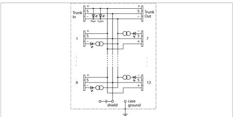
The junction box is designed for fieldbus Note: It must be ensured that there is suffisystems acc. to IEC 61158-2, i.e. it is suited for both FOUNDATION™ fieldbus and PROFIBUS-PA. When connected to a suitable ing via the housing's M5 x 1 grounding bold. power supply unit, it can also be used in Ex
