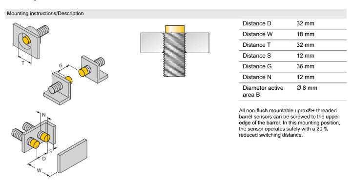
Mounting clamp for threaded barrel sensors, with dead-stop; material: PA6
