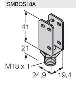
3069721 Mounting bracket, stainless steel, for 18 mm thread
