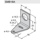
Mounting bracket, rectangular, stainless steel, for sensors with 18 mm thread
