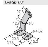
3067467 Mounting bracket, stainless steel, for 18 mm thread
