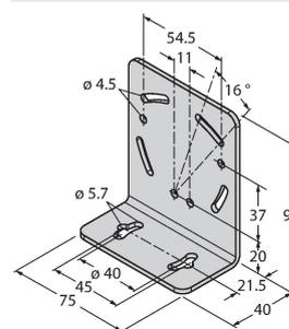
Mounting bracket, rectangular, stainless steel, for sensors of the LTF series
