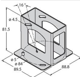
Protective housing, stainless steel, for sensors of the LTF series
