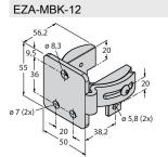
Mounting bracket, steel, blackfinished, for EZ-ARRAY and EZ-SCREEN standard and cascade 14 &
