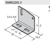
Mounting bracket, stainless steel, rectangular, for Q20 3,2 x 12,6 (2x)
