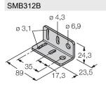
Mounting bracket, stainless steel, for MINI-BEAM NAMUR
