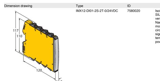
Isolating switching amplifier, 2-channel; SIL2 acc. to IEC 61508; Ex-proof version; 2 transistor outputs; input Namur signal; ON/OFF switchable monitoring of wire-break and short-circuit; toggle between NO/NC mode; signal doubling; removable screw terminals; 12.5 mm wide; 24 VDC power supply
