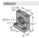
3052521 Mounting bracket, PBT black, for sensors with 30 mm thread, rotatable
