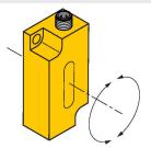
Adjusting the measuring range via TX1-Q20L60 teach adaptor
