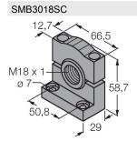
3053952 Mounting bracket, PTB black, for sensors with 18 mm thread
