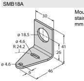
3033200 Mounting bracket, rectangular, stainless steel, for sensors with 18 mm thread
