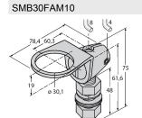
Mounting bracket, stainless steel, for M10 x 1.5 thread, thread length 30 mm
