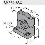
3053952 Mounting bracket, PTB black, for sensors with 18 mm thread
