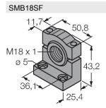
3052519 Mounting bracket, PBT black, for sensors with 18 mm thread, rotatable
