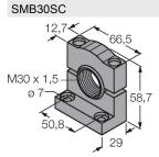
3052521 Mounting bracket, PBT black, for sensors with 30 mm thread, rotatable
