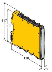
7580020 Isolating switching amplifier, 2-channel; SIL2 acc. to IEC 61508; Ex-proof version; 2 transistor outputs; input Namur signal; ON/OFF switchable monitoring of wire-break and short-circuit; toggle between NO/NC mode; signal doubling; removable screw terminals; 12.5 mm wide; 24 VDC power supply
