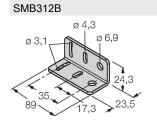
Mounting bracket, stainless steel, for MINI-BEAM NAMUR
