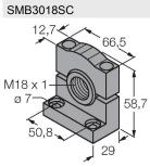
Mounting bracket, PTB black, for sensors with 18 mm thread
