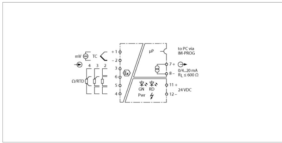
The temperature measuring amplifier IM34-11Ex-Ci/24VDC is designed to evaluate the temperature-dependent changes of Ni100/Pt100 RTDs, thermocouples types B, E, J, K, L, N, R, S and T or low voltages in a range of -160...+160 mV and to output them as temperature-linear current signals.
