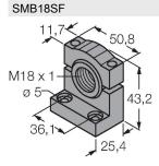
Mounting bracket, PBT black, for sensors with 18 mm thread, rotatable
