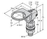
Mounting bracket, stainless steel, for M10 x 1.5 thread, thread length 30 mm
