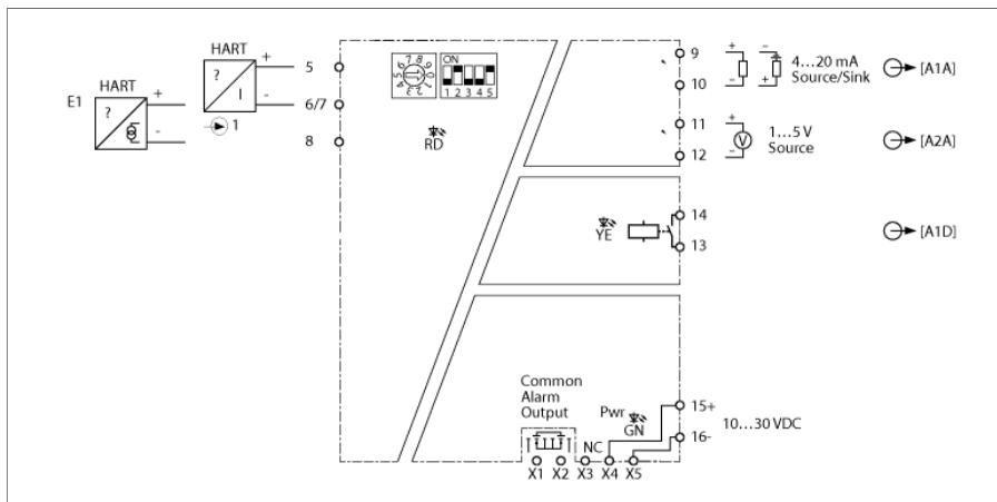
The IM12-AI01-1I-1IU1R-H... isolating transducers transmit the analog measured signal in a galvanically isolated manner. In addition, the devices monitor the input signals for exceeding or falling below an adjustable limit value. The devices are suitable for operation in Zone 2. Passive 2-wire transducers, as well as active and passive HART transmitters, can be used on the devices.
