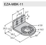
3071470 Mounting bracket, steel, blackfinished, for EZ-ARRAY and EZ-SCREEN standard and cascade 14 & 30 mm
