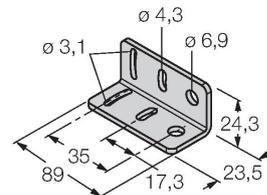
Mounting bracket, stainless steel, for MINI-BEAM NAMUR
