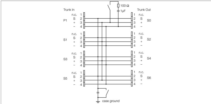
The 6-channel junction box JBBS-48-T615/3G is designed for PROFIBUS-PA systems.
