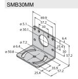
Mounting bracket, rectangular, stainless steel, for sensors with 30 mm thread, wide holes for accurate alignment
