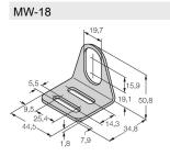
Mounting bracket for threaded barrel sensors; material: Stainless steel A2 1.4301 (AISI 304)
