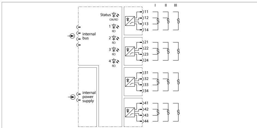
The input module TI41-N is used for the connection of the 2, 3 and 4-wire temperature probes Pt100, Ni100, Cu50 and Cu100.
