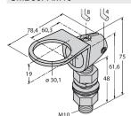
Mounting bracket, stainless steel, for M10 x 1.5 thread, thread length 30 mm
