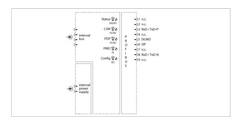
The GDP-NI gateway serves to connect the *excom*® system to PROFIBUS-DP networks. Connection to the PROFIBUS-DP is established via optical fibers or copper cables. When using optical fibers for data transmission, an optocoupler pair must be installed between wired and optical PROFIBUS.
