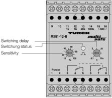
The 1-channel level control MS91-12-R monitors and regulates conductive liquid levels (II). As a dual level regulator, it can be used to control pumps and solenoid valves (I). As monitoring device it is designed for run-dry or over flow protection.
