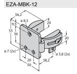
Mounting bracket, steel, blackfinished, for EZ-ARRAY and EZ-SCREEN standard and cascade 14 & 30 mm
