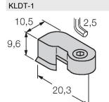
Clamping piece for mounting magnetic field sensors on dovetail groove cylinders; clamping width:
