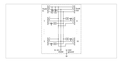
The junction box is designed for fieldbus systems acc. to IEC 61158-2, i.e. it is suited for both FOUNDATION™ fieldbus and PROFIBUS-PA. When connected to a suitable power supply unit, it can also be used in Ex applications.
