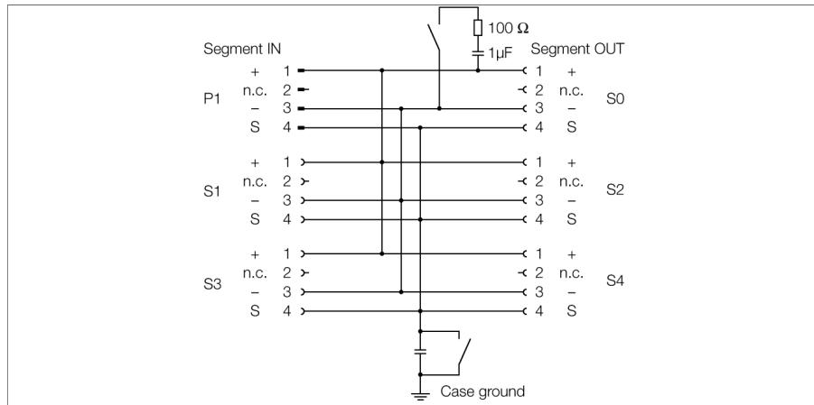
The 4-channel Ex junction box JBBS-48-E413/EX is designed for PROFIBUS-PA systems.
