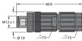
Field-wireable male connector, M12 × 1, straight, 4-pin, push-in connection, cable feedthrough 4.0 to 8.0 mm, core cross-section/terminal capacity 0.14 to 0.75 mm<sup>2</sup>, plastic housing, metal retaining screw
