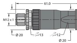
Field-wireable male connector, M12 × 1, straight, 4-pin, screw terminal connection, cable feedthrough 4.0 to 8.0 mm, core cross-section/terminal capacity 0.25 to 1.5 mm<sup>2</sup>, plastic housing, metal retaining screw
