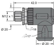
Field-wireable male connector, M12 × 1, angled, 4-pin, screw terminal connection, cable feedthrough 4.0 to 8.0 mm, core cross-section/terminal capacity 0.25 to 1.5 mm<sup>2</sup>, plastic housing, metal retaining screw
