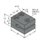
Fixing clamp; material mounting block: Anodized aluminium
