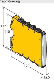
IMX12-DI01-2S-2T-0/24VDC 7580020 Isolating switching amplifier, 2-channel; SIL2 acc. to IEC 61508; Ex-proof version; 2 transistor outputs; input Namur signal; ON/OFF switchable monitoring of wire-break and shortcircuit; toggle between NO/NC mode; signal doubling; removable screw terminals; 12.5 mm wide; 24 VDC power supply
