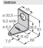
3032723 Mounting bracket, rectangular, stainless steel, for sensors with 30mm thread
