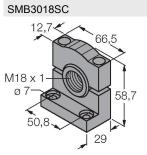
Mounting bracket, PTB black, for sensors with 18 mm thread
