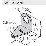
Mounting bracket; material VA 1.4401, for Q12 & M12 series
