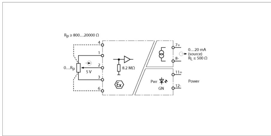
The 1-channel potentiometer amplifier IM36-11EX-I/24VDC is designed to transmit signals from 3 or 5-wire potentiometers galvanically isolated from the Ex area to the non-Ex area and to converted them into normalized 0...20 mA analog signals. The resistance value of the wiper contact, ranging from 0  $\Omega$  to the nominal resistance value (final value) of the potentiometer, is detected and linearly processed.
