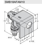
3012558 Mounting bracket, material VA 1.4401, for M10 x 1.5 thread, thread length 18 mm
