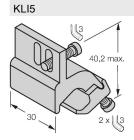
6971802 Mounting bracket for mounting magnetic field sensors on profile cylinders; cylinder diameter: 32...50 mm; material: Aluminum
