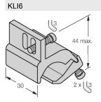
6971805 Mounting bracket for mounting magnetic field sensors on profile cylinders; cylinder diameter: 50...100 mm; material: Aluminum
