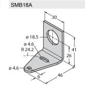
3033200 Mounting bracket, rectangular, stainless steel, for sensors with 18 mm thread
