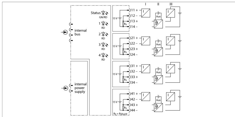
The input module AI401Ex is used for the connection of 2-wire transducers (active input = source mode / transducer passive) or 4-wire transducers (passive input = sink mode / transducer active).
