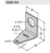
Mounting bracket, rectangular, stainless steel, for sensors with 18 mm thread
